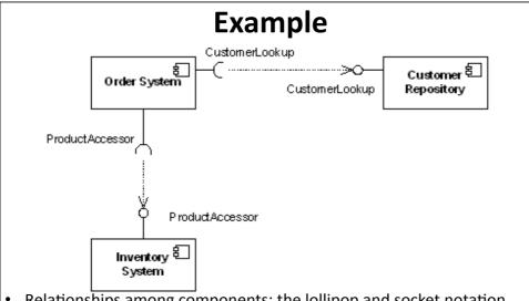
Relationships among components: the lollipop and socket notation can also include a dependency arrow (as used in the class diagram).
