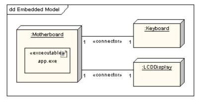
Deployment diagram for part of an embedded system, depicting an executable artifact as being contained by the motherboard node
